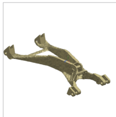
Based on previously defined loads and boundaries solidThinking Inspire calculates the optimal structure.
