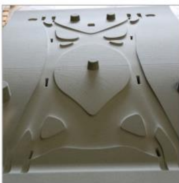
3D printed sand form for casting, made by voxeljet.
