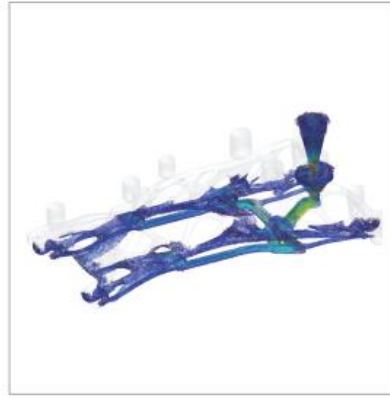
Velocities of casting process in Click2Cast simulation.
